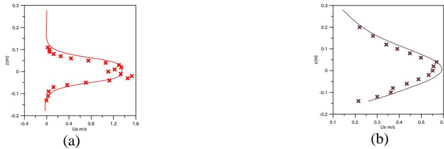
Figure 1. Vertical distribution of mean velocities along the jet axis at distance 0.1 (a) and 0.7 (b) m from propeller. Curves are VH-PU model computations, symbols are lab measurements (Schokking 2002).
