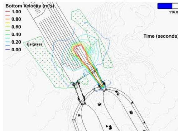
Figure 3. Bottom velocities generated by Issaquah-class ferry during landing at Port Townsend ferry terminal, Puget Sound, WA at simulation time = 116 sec. Also shown are bottom elevation contours, eelgrass locations and terminal and vessel locations.
