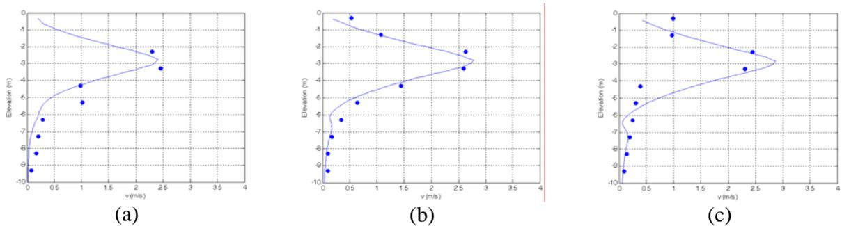
Figure 2. Vertical distribution of velocities along the jet axis at time 1.0 (a), 3.0 (b) and 5.0 (c) seconds. Curves are VH-PU model computations, symbols are field measurements (2-second averages).
