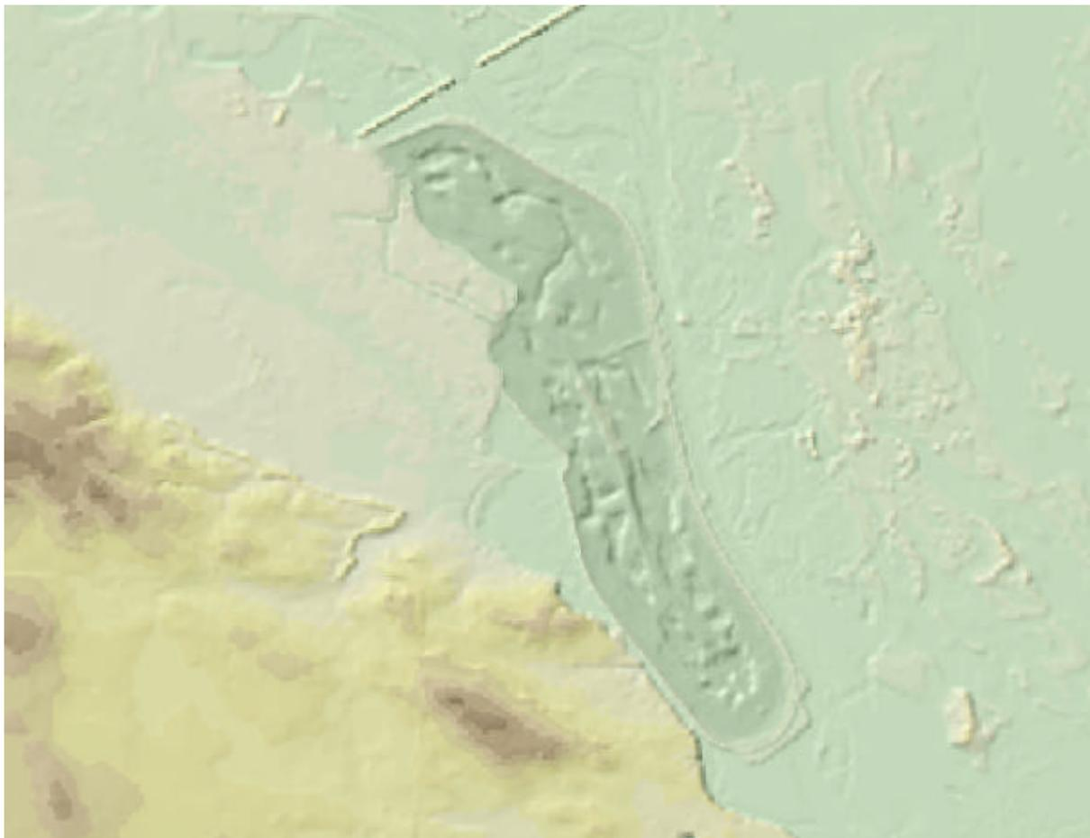
Fig. 1.4. The result of integration of the model of the Exclusion Zone surface relief created upon the data of map with scale 1:10 000 with the model of the Cooling Pond bottom relief
